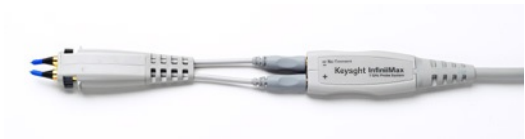
Figure 25 1134A/B Probe Amplifier and E2675A/B Differential Browser Probe Head
